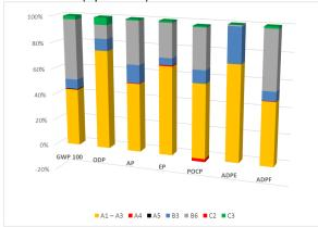
Module A1-3 has a significant influence on the CML results due to the material pre-processes. This module is dominant with regard to the Ozone Depletion Potential (ODP), Acidification Potential for soil and water (AP), Eutrophication Potential (EP), Photochemical Ozone Creation Potential (POCP) and the Abiotic Depletion Potential for Elements (ADPE). Especially the electronic components in the operator as the gear motor and the power supply are mainly responsible for this.
