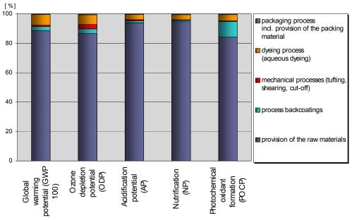
Figure 6: Relative contributions of different partial processes of production to the environmental impacts during product manufacture
