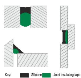
The adhesion of more than two sides can be performed with the aid of joint insulating tape.
